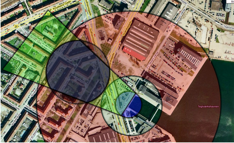
Fig. 8.3 Distance inaccuracy is larger than the bearing inaccuracy
