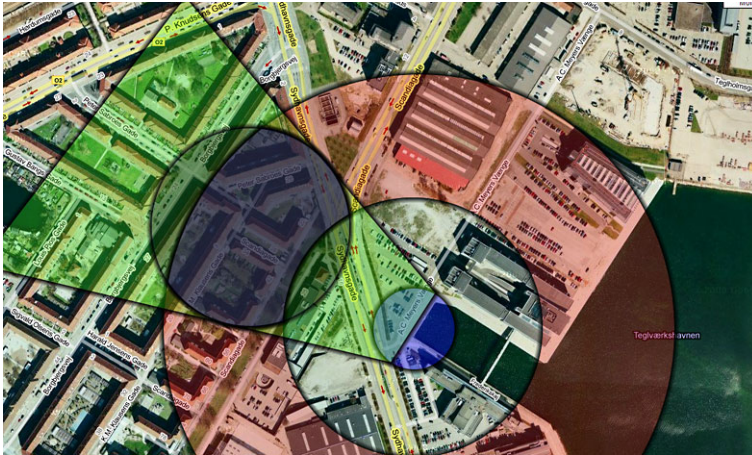
Fig. 8.4 Distance inaccuracy is smaller than the bearing inaccuracy
